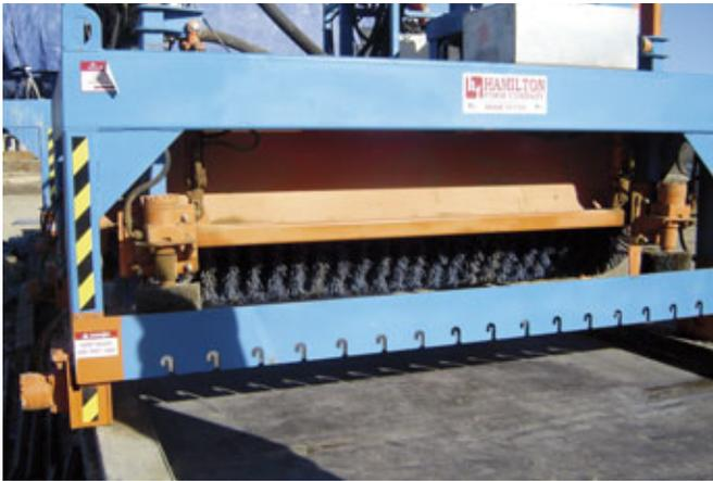
Hydraulic double brushes allow the form side walls and flat deck surfaces to be cleaned in a single pass.
