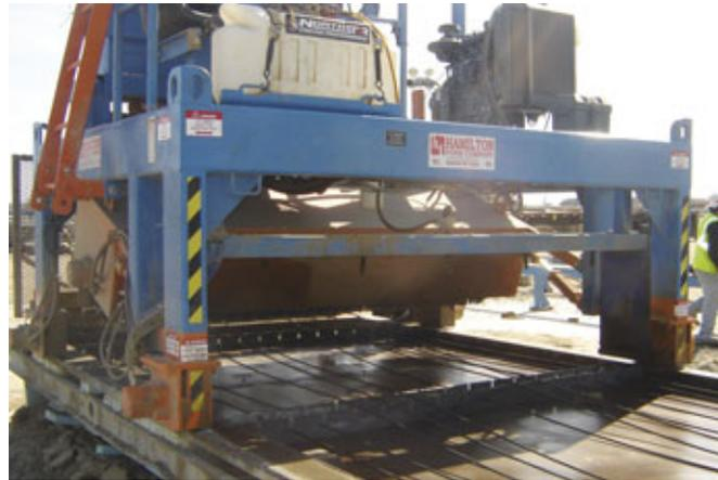
As many as 8-to-10 prestressing strands are pulled and dropped simultaneously into each header along the 400-foot bed.
