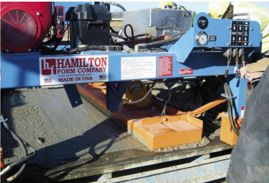
A high frequency vibrating screed raises and lowers hydraulically.
