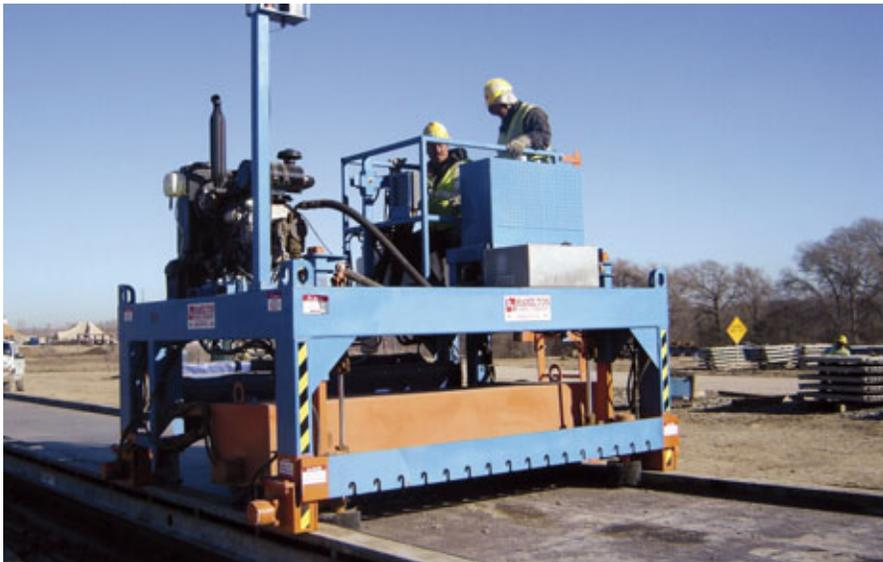
Hamilton Form designed and produced this multitasking Form Cleaning, Sprayer, Strand Puller Machine to help prepare beds for casting.
