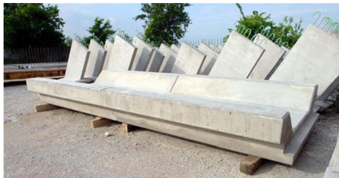
A total of 900 custom-made precast sections, including 6,500-plus feet of 9-ft. x 10-ft. trench panels, supplied by Speed Fab-Crete will help create a 'green' deck park surmounting Dallas' concrete jungle.
