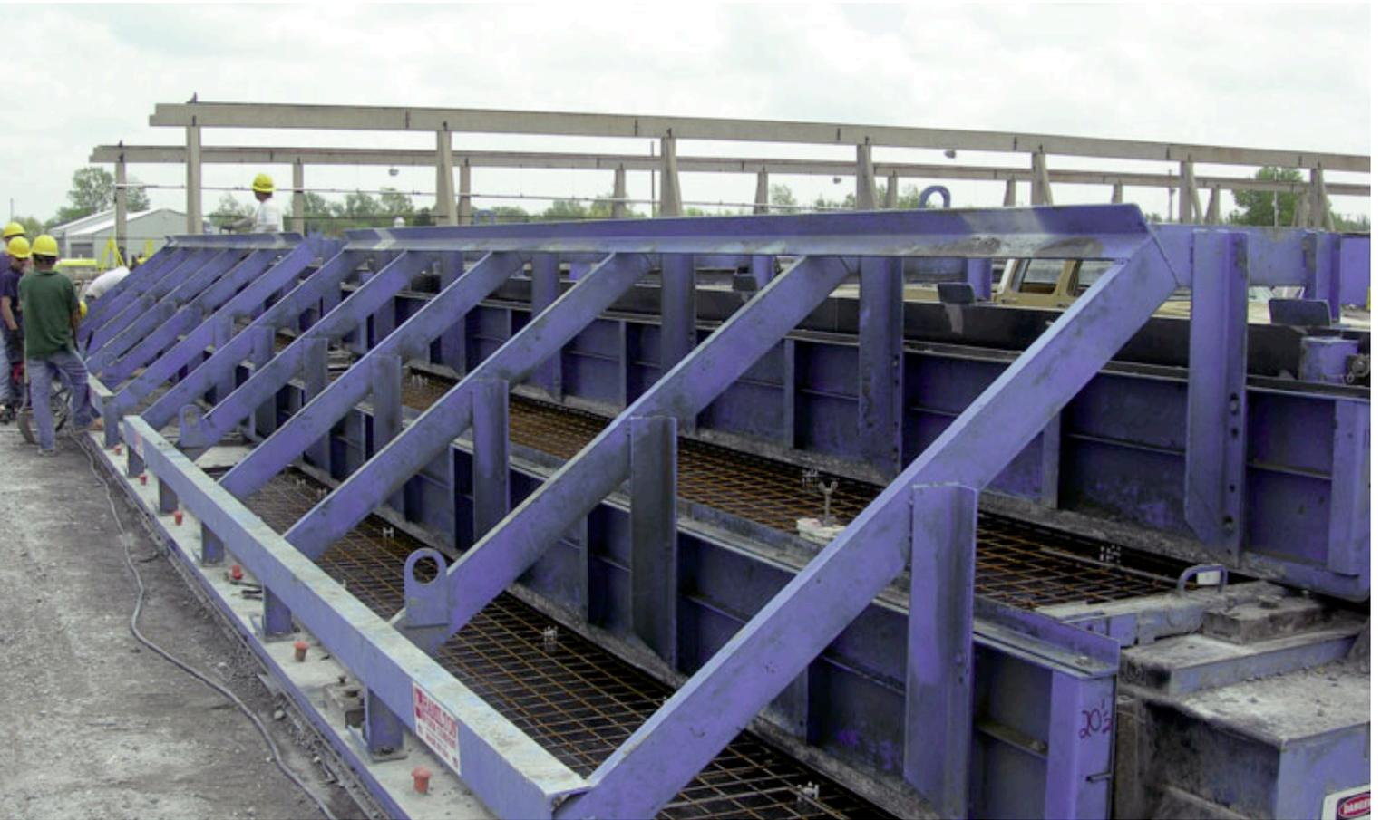
*Double L Riser for Intrust Arena at Prestressed Concrete, Inc*
