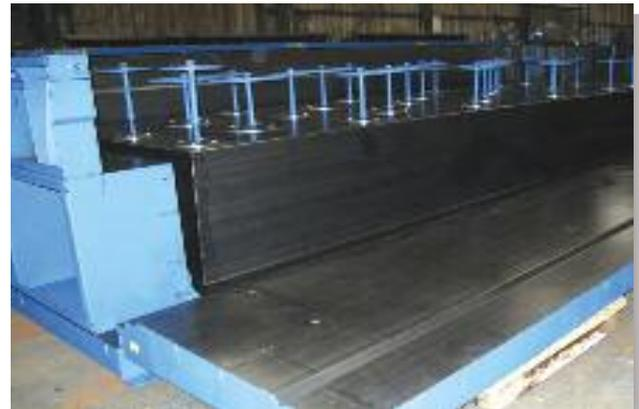
Sideforms pivot open for stripping.
