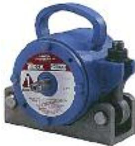
An easy and convenient method for applying vibration is with a **MACH™ 1 External Vibrator**. The design of the MACH vibrator has proven to be durable and trouble-free. It requires no bearings and only has three moving parts. The MACH Vibrator can be attached to a bracket on the outside of the form, used with Vibrotrack or used with vibratory screeds.
