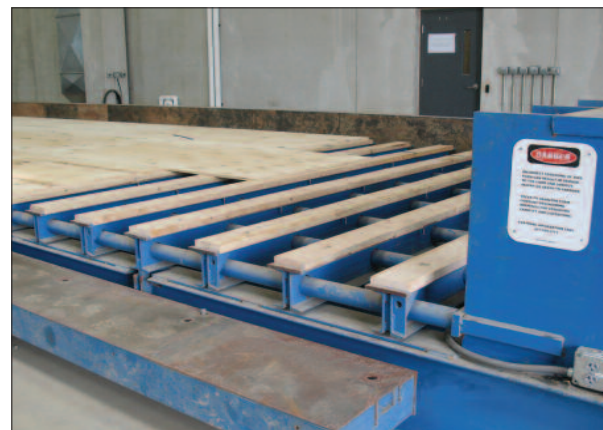
Hamilton Form's self-stressing architectural casting frame is installed, then topped with a wood deck and architectural finish.
