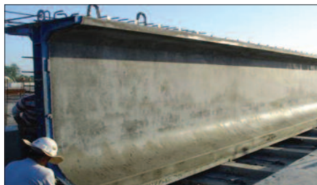
A single sideform with no filler produces beams with no noticeable seams.
