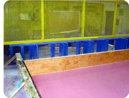
*Hamilton Form recently delivered a 16'-0" self-stressing casting table frame to Shockey Precast Group. The frame is topped with plywood and fiberglass for a smooth, seamless casting surface.*
