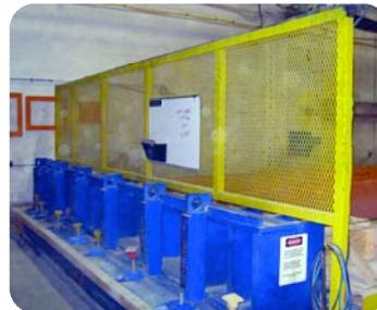
*Sliding jacking plates adjust for different strand patterns to save set up time.*
