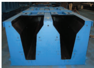
Dual line median barrier form with hanging block-out assemblies.
