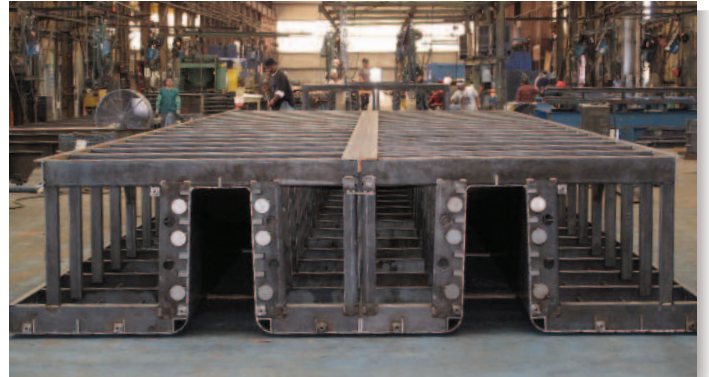
The form was split at centerline for shipping and handling considerations.
