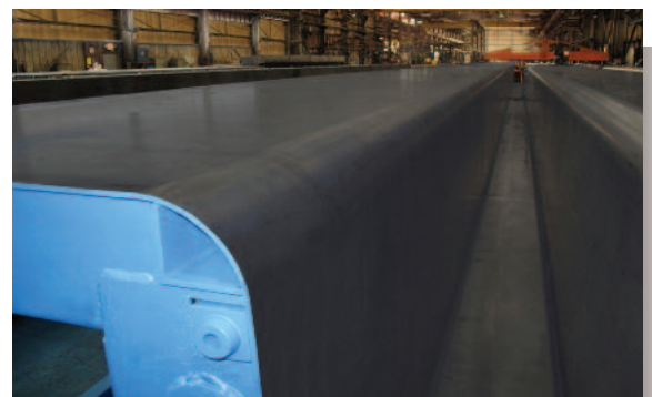
A four-inch radius forms the stem to deck transition.
