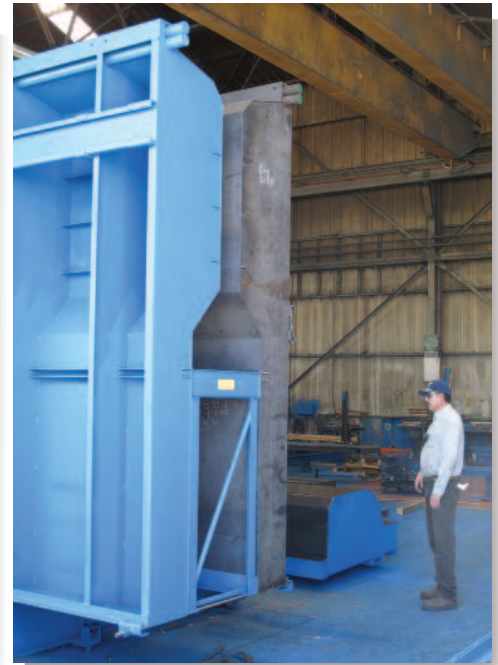
Haunch girder sideforms with self-stressing bars.
