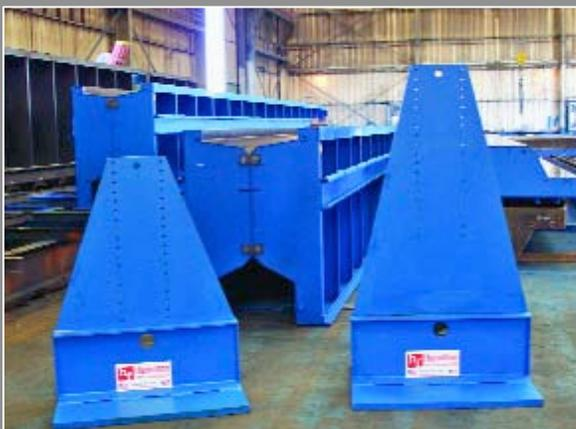
*These internal strand hold ups were designed to be used in the production of TXDOT bridge girders. The base plate distributes the downward force evenly over the soffit. The vertical plate has two rows of holes that are fitted with strand rollers. The vertical plate can be shimmed for added adjustability. Two sizes of hold ups were built so that the customer could accommodate G38 through G78 girders.*
