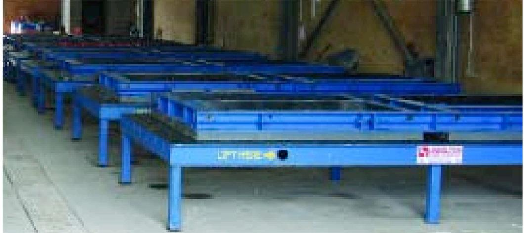
Over the past few years, Hamilton Form has built over forty retaining wall forms for Atlantic Industries Limited (AIL). AIL is a major supplier of custom infrastructure solutions. The forms made by Hamilton Form are used to cast retaining wall panels for AIL's Vist-A-Wall™ MSE Structural Wall Systems. This wall system is used in bridge abutments, embankments and retaining walls across Canada, the U.S., and for projects in the Caribbean and Australia.
