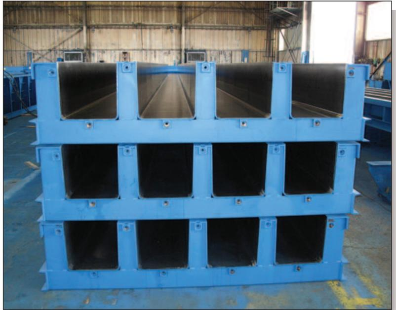
Depending on the pile size, a dual, triple, or even quad-line form may be most cost-effective.
