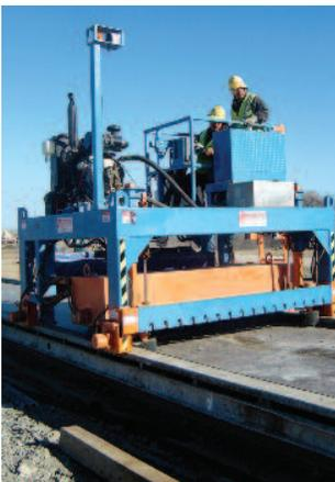
Hamilton Form Utility/Casting Machines mechanize precast/prestressed concrete production making the process more consistent, shorten set-up time, decrease production costs and help improve product quality.
