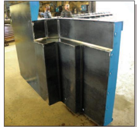
**A** hanging back pan is attached to the top of the form to create the top ledge. A mat is used on the flat reveal area on each side of the fluted center to create a bush hammered finish. A removable riser with integral top ties form the holes at the back of the product where protruding rebar ties into the retaining wall.
