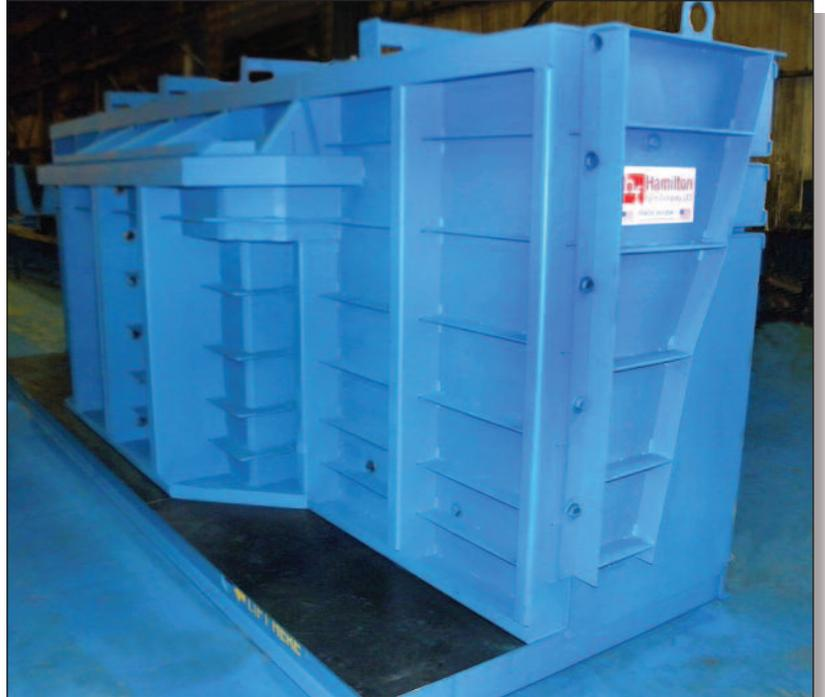
Precast concrete plays prominently in bringing the design concept to life. The MSE retaining walls, supplied by Tricon Precast in Houston, feature a special decorative coping that ties into the design theme. The coping sits at the top of a precast “winged” column and has a stepped design on the face of the panel that creates depth and shadows. The design is unique, and so is the form used to produce the coping.
