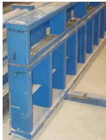
24" side form with 12" riser anchored with magnets.
