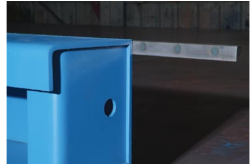
Magnets are embedded in holes within a steel chamfer with no open grooves to fill with concrete.
